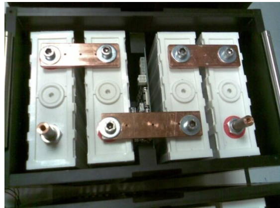
Figure 19: Inside view of the 100 Ah module
