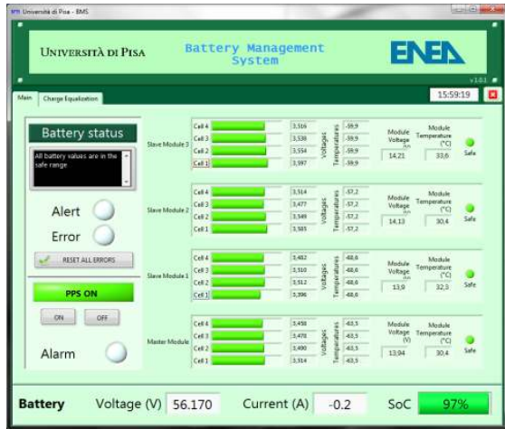
Figure 17: BMS user interface
