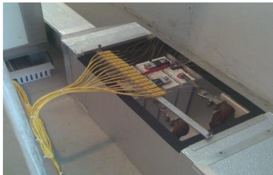
Figure 10: The cells with the thermal sensors inside the test section
