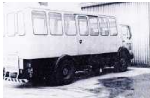
(b) British Pavement Deflection Data Logging Equipment. Mark II.
