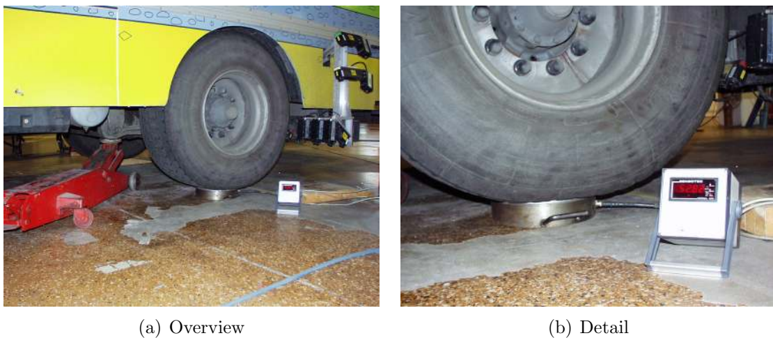
Figure 3.9: Calibration of the left wheel force transducer.
