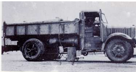
(a) The first Lacroix prototype (1956). This version is built on a Willème S. 10 truck.
