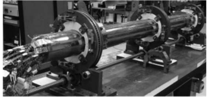
Fig. 4. Assembly of two dipole coils with protection heaters and ground insulation.
