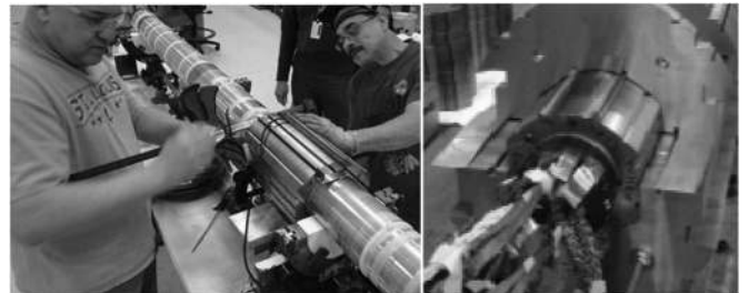
Fig. 5. Installation of collar blocks around coils (left), collared coil inside iron yoke (right).
