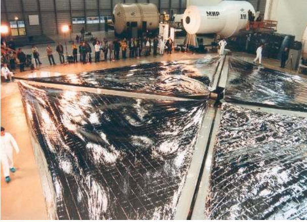
Figure 2: The CFRP booms confirmed their capabilities during the on-ground verification of the Solar Sail project. End of 1999, DLR site Cologne.
