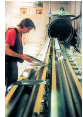
Figure 9: Manufacturing of the CFRP booms was carried out by use of ultra thin-walled CFRP prepregs via a classical prepreg/autoclave technique in conjunction with a modular CFRP tooling concept. After curing, two half-shells were bonded by use of an adhesive.
