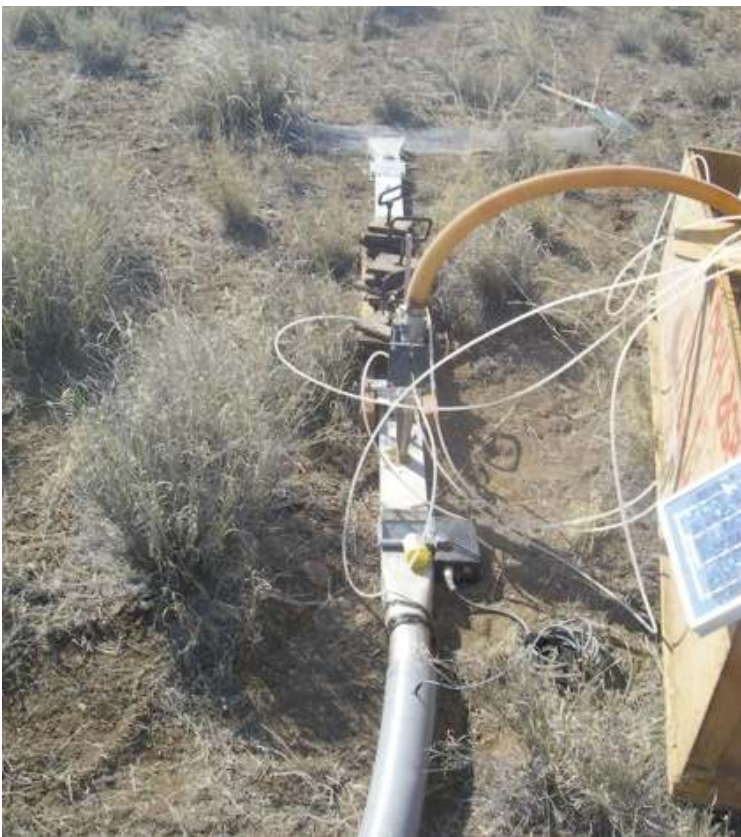
418 Fig. 7 The micro wind tunnel was highly suitable to deployment in a grassed rangeland site because its small 419 footprint could fit between grass clumps
