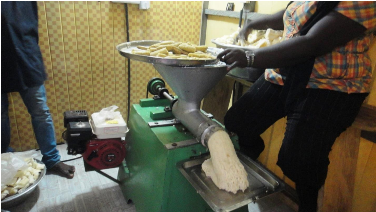
Fig. 6: Fufu Pounding Machine.
