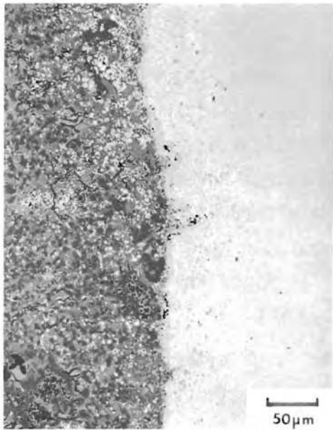
FIGURE 3.B-7. Microstructure of Hot Pressed SPC-4E Pellets in TiO_2 (run no. 2 right and 11 on left)
