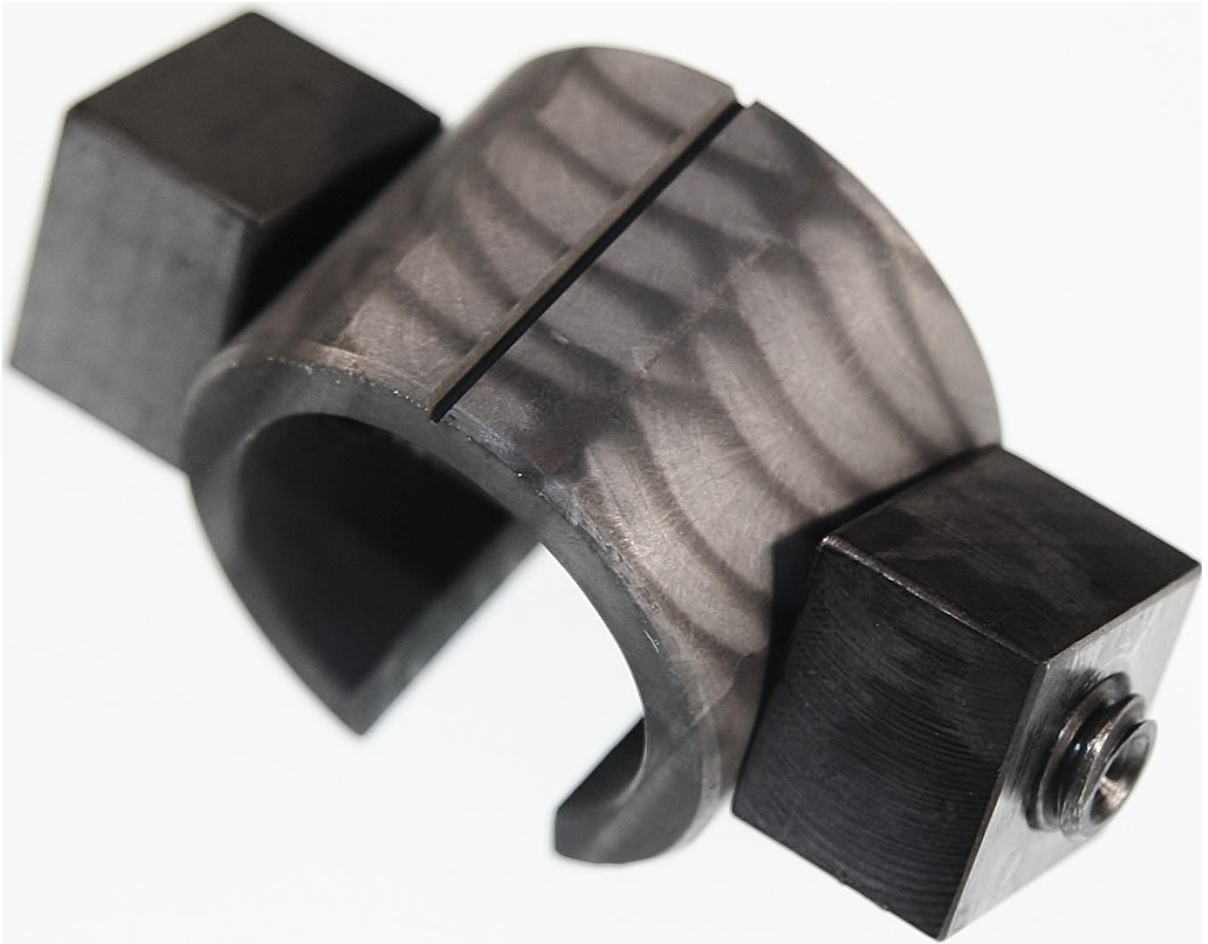
Figure 23. A notched C-Ring reheat cracking test specimen showing the correct placement of the notch traversing several overlapping weld bead passes in a narrow gap weld deposit, ~4X.
