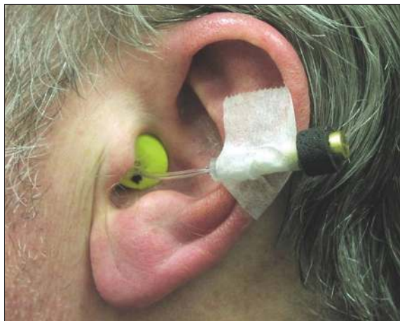
Figure 3: Earplug with probe, with brass nipple inserted to seal the probe at the distal end
