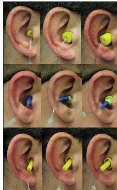
Figure 4: Examples of good (left), degraded (middle), and unacceptable (right) fits for Classic (top), Push-Ins (middle), and UltraFit (bottom) earplugs
