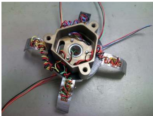
(c) Supporting structure of the feet with strain gauges glued to the claws
