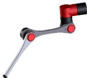
Figure 3.2: The kinematic structure of a leg
