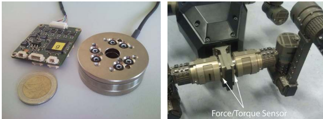
(a) ATI Industrial Automation force/torque sensor Mini45-E together with custom-designed force/torque sensor board (b) Force/torque sensor mounting between body and leg on the real robot
