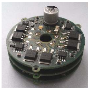
(b) Photo of the actuator electronic stack
