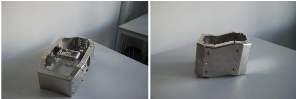
Figure 3.12: Body design. Left: main body frame, right: front body frame.
