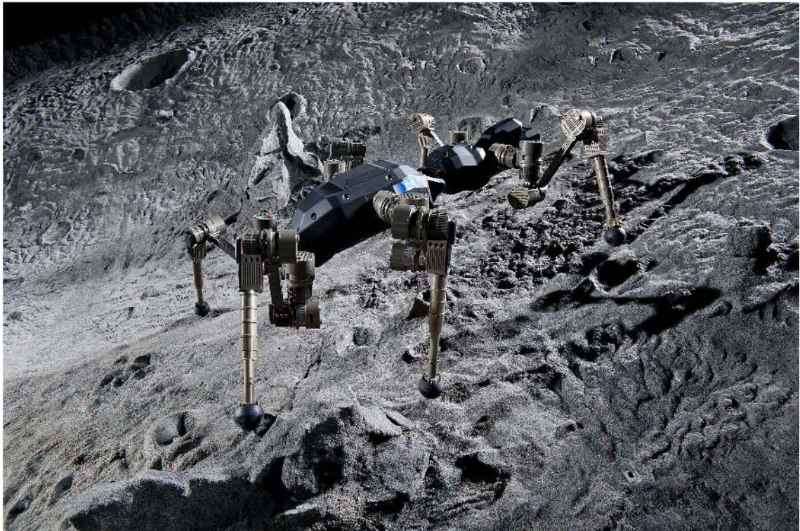
Figure 3.1: Photo of the fully functional SpaceClimber robot in the artificial DFKI moon crater environment
