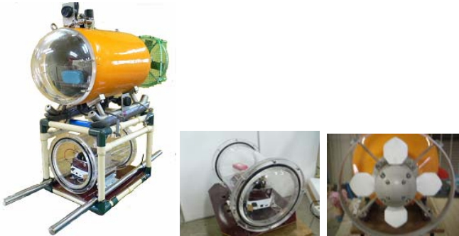
Fig.3 UROV system, camera housing and propeller blade
