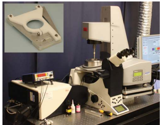
FIG. 1. Photograph of the confocal rheometer. The base plate of an Anton Paar MCR301 rheometer is replaced with a metal cup. Optical access for a Leica SP5 confocal microscope is provided by a glass coverslip mounted in the cup, which serves as the rheometer bottom plate. The field of view of the microscope can be changed by moving the rheometer on a manual three-axis translation stage. The inset shows the device that clamps the cup to the microscope stand to reduce vibrations.
