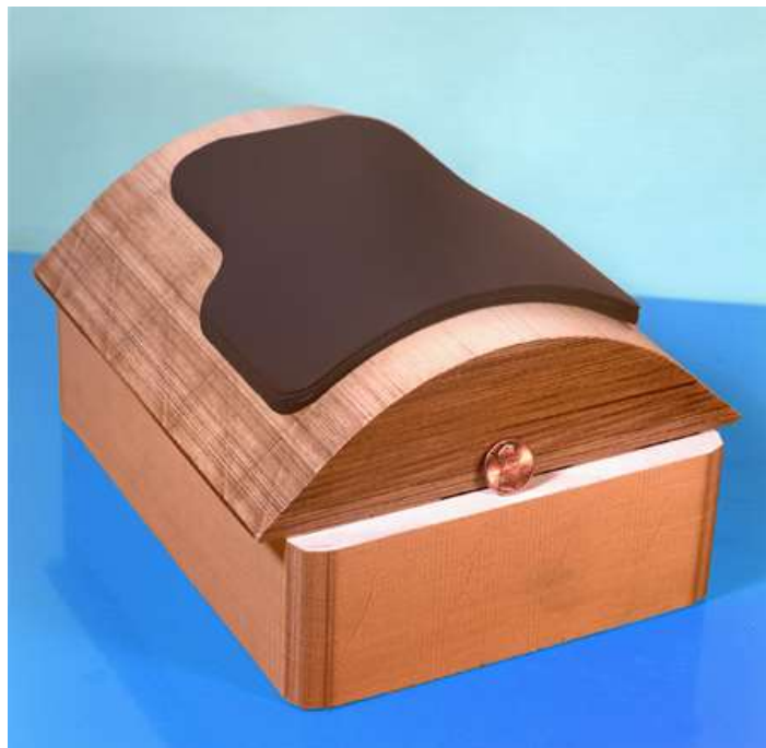
Figure 12: Curved layer, monolithic SiC body armor panel, immediately after LOM processing. The piece has been fully decubed and placed back on the LOM-paper mandrel for illustration. Notice the smooth surface and lack of stair steps.
