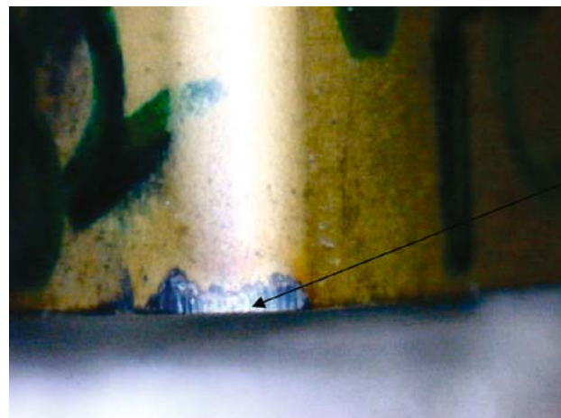
Fig. 2 Artificial flank wear created by EDM process
