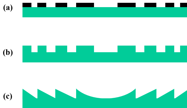
Fig. 1.1: (a) Fresnel Zone Plate (FZP). (b) Phase Zone Plate (PZP) or "binary" lens. (c) Phase Fresnel Lens (PFL).
