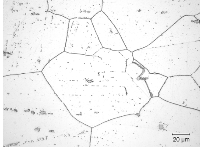
Fig. 2 Age-hardened microstructure of 282 alloy
