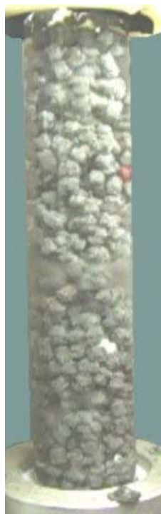
Figure 5: Fluidized bed of capsules during testing showing tracer particles
