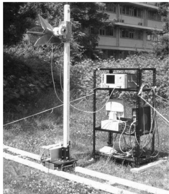
Fig. 1. Configuration of the broadband ground-based polarimetric SAR system. (a) A schematic and (b) photograph of the developed system as built.
