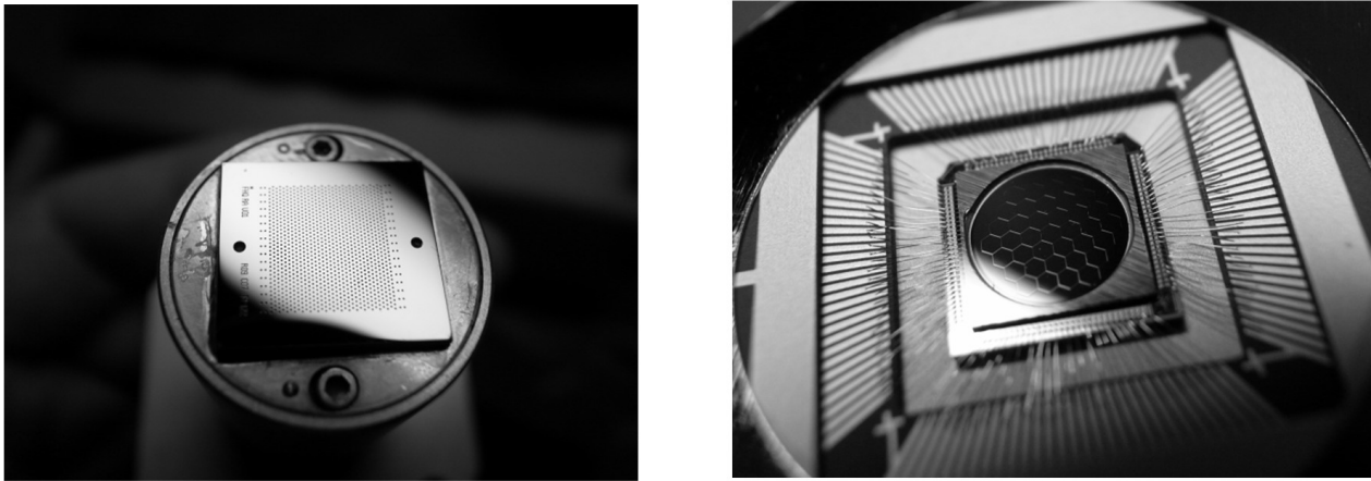
Figure 2. Left: Two-dimensional fiber array from FiberGuide Industries. The fiber pitch is 250 \mu\text{m} . Right: Segmented Deformable Mirror from IRIS AO. The pitch between adjacent segments is 606.2 \mu\text{m} including a 4 \mu\text{m} gap.
