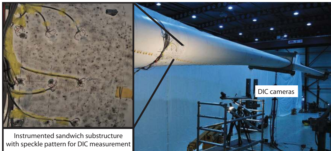
Figure 5. DIC setup and the instrumented region of interest
