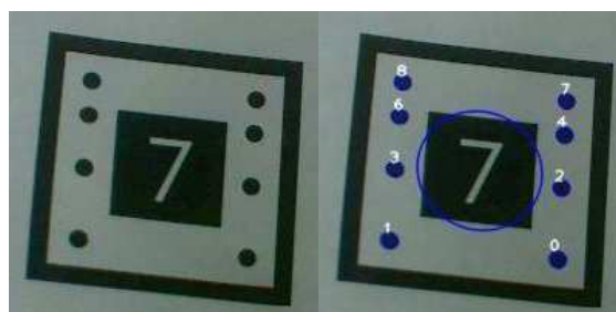
Fig. 5. Designed underwater pattern for P-SURO AUV.
