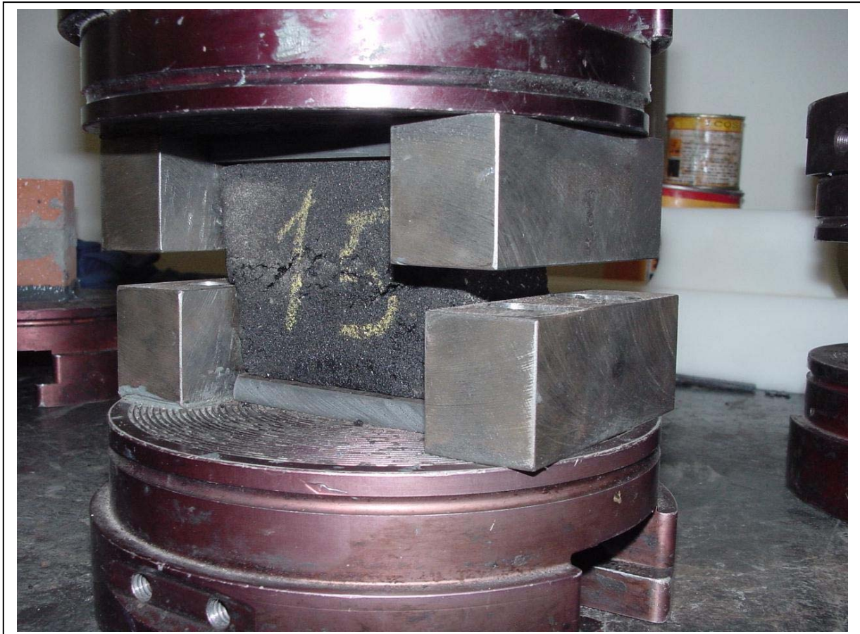
Figure 4 – Test specimen used in tensile adhesion test glued to the machine platens
