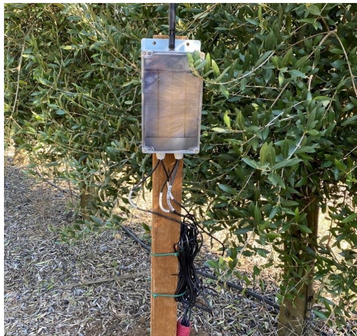
Figure 8. Communication node with connected soil moisture sensors.
