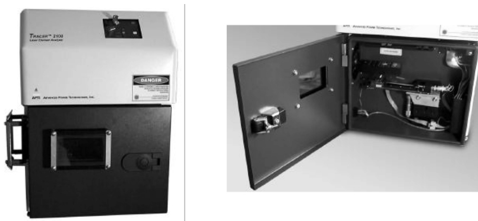
Fig. 1. TRACER™ 2100 instrument and the inside of the sample chamber showing the automated multi-sample positioning stage.
