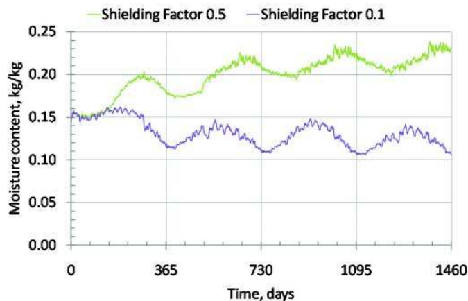
Figure 8 Moisture content in the beam end with shielding factor of 0.1 and 0.5 for an insulated wall with a 300 mm (11.81 in.) gap in the insulation towards the floor.
