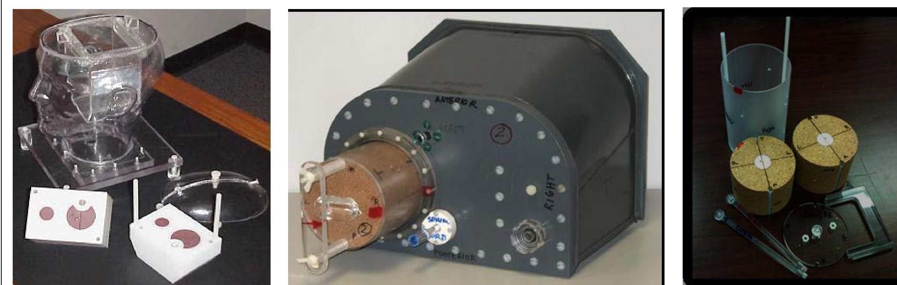
Figure 1: The IROC-H head and neck phantom (left) and lung phantom (center) used in the benchmarking study are shown. The head and neck phantom is shown with the dosimetry insert removed and opened, revealing a transverse view of the mock PTV (crescent shape), secondary PTV (larger of two cylinders) and OAR (small cylinder). The insert to the lung phantom (right) is shown along with removable rods for TLD that are placed at locations consistent with the heart and spine.
