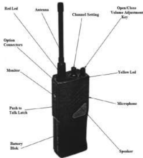
Figure 2. Constituent parts of the radio
