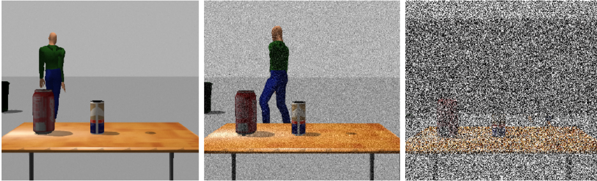
Fig. 3.5 Demonstration of the effect of Gaussian noise modelling on simulated IMPEP camera image quality. Gaussian noise with zero-mean was applied in all cases: from left to right, the standard deviations are 0.007, 0.1 and 1, respectively.
