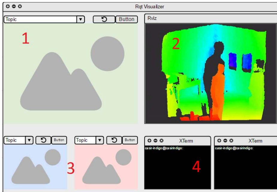
Fig. 3.13 Mockup of the first version of the rqt -based interface. Each frame in the interface in this version, all of which with predefined fixed sizes in the dashboard, was preconfigured to display information as follows: (1) is the main camera visualisation frame; (2) is the main processed data (e.g. 3D reconstructions, signal waveforms, etc.) visualisation frame; (3) contains two secondary frames for camera (or related data, such as depth maps, etc.) visualisation; (4) contains frames for two support terminals. Note, however, that all of these frames are reconfigurable to display whatever is needed by the user/developer on the fly.
