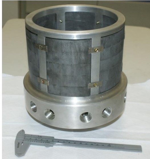
Figure 59: The stator of the rotary thermomagnetic motor, with the Gd_{4.7}Nd_{0.3}Si_4 magnetic material plates mounted.
