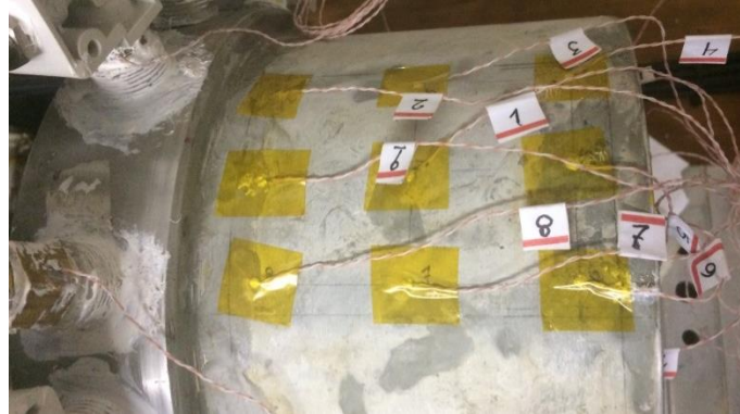
Figure 63: The experimental measurement of the temperature developed in the magnetic material plate. To the left side can be seen the nylon plug connections and the control valve.
