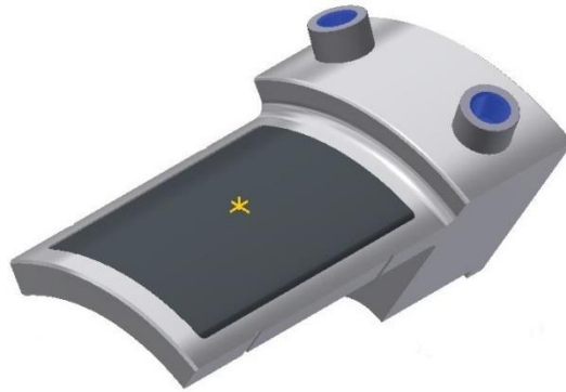
Figure 57: The model of the magnetic material plate and support structure used for the CFD simulations.
