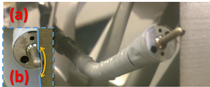
Figure 15: View of the continuum robot within the mock-up aero engine when machining (blending) a virtual defect on an aerofoil;
