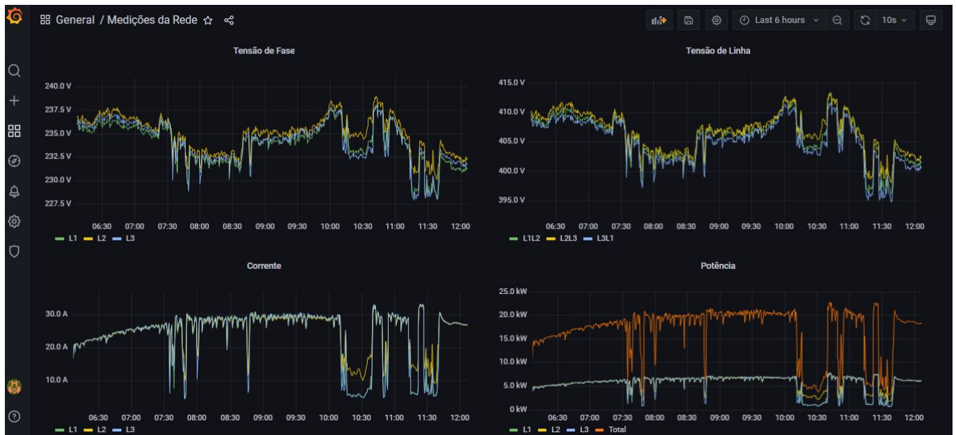
Figure 18. AC-Grid measurements for the solar power plant.
