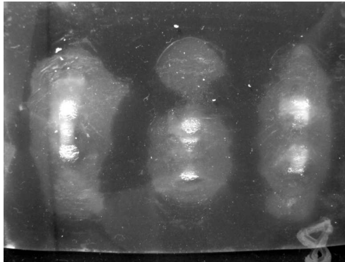
Figure 2: Results of three tests of a 3SP sample under the following conditions: no surface treatment, low dermal stiffness (polyurethane), 50 mm/s shear speed, and 6 N normal load. The light-colored regions are blisters, while the bright white regions indicated significant surface damage
