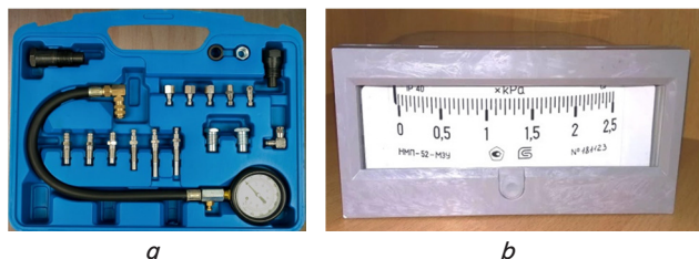
Fig. 1. Equipment for determining the cylinder-piston group parameters: a – HS-A1019; b – NMP-52
