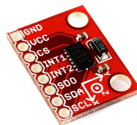
Fig. 3. The triaxial ADXL345 MEMS- accelerometer
