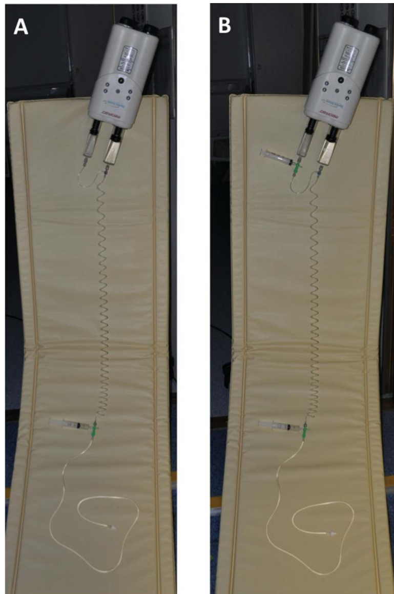
Figure 2 A dual-head power injector and tubing set-up for a perfusion CMR in the case of the dual-head power injector with and without a “pause” function (A and B respectively). Please see the text for details.
