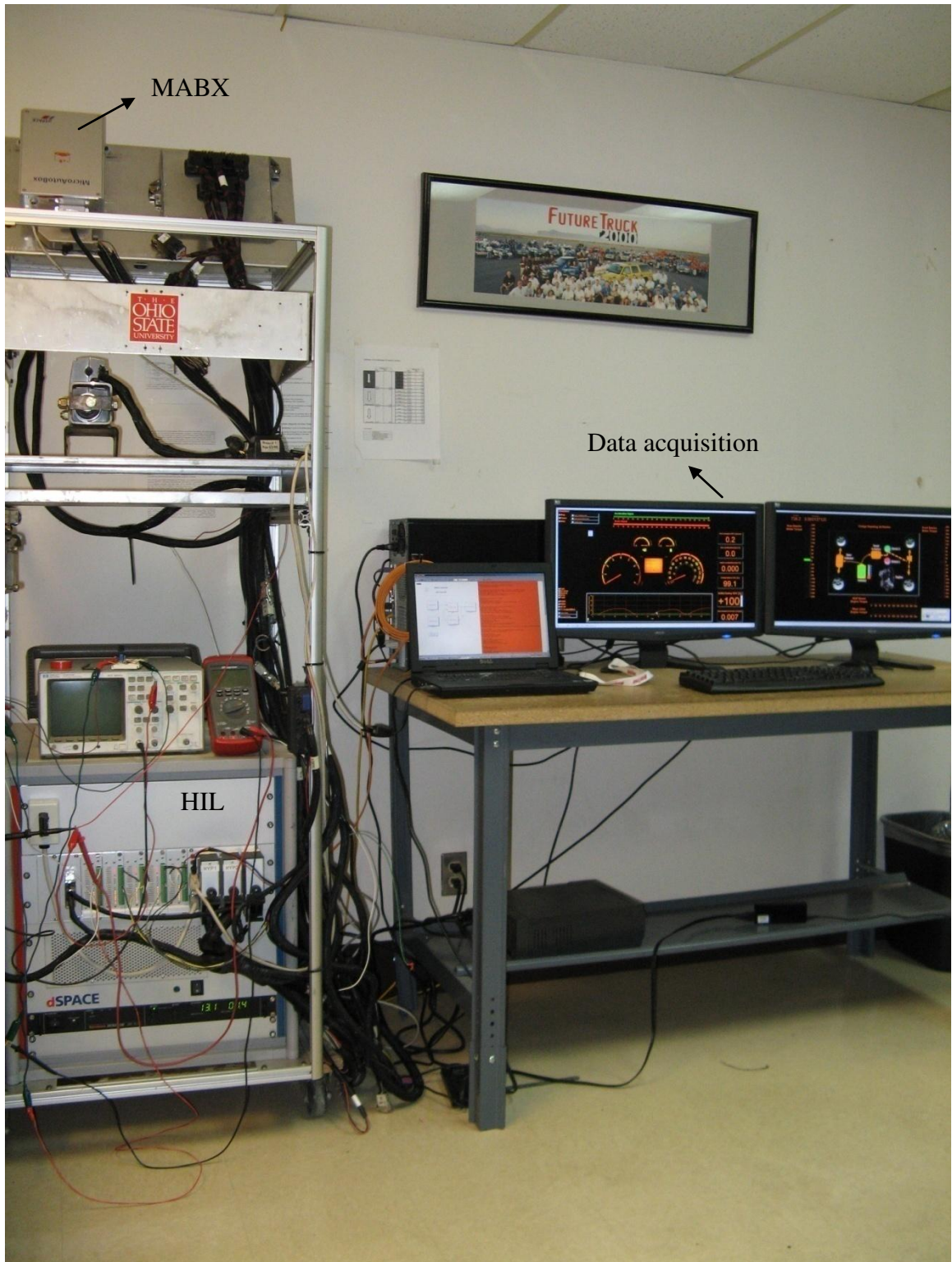
Figure 61 Real time simulation set-up showing the main components.
