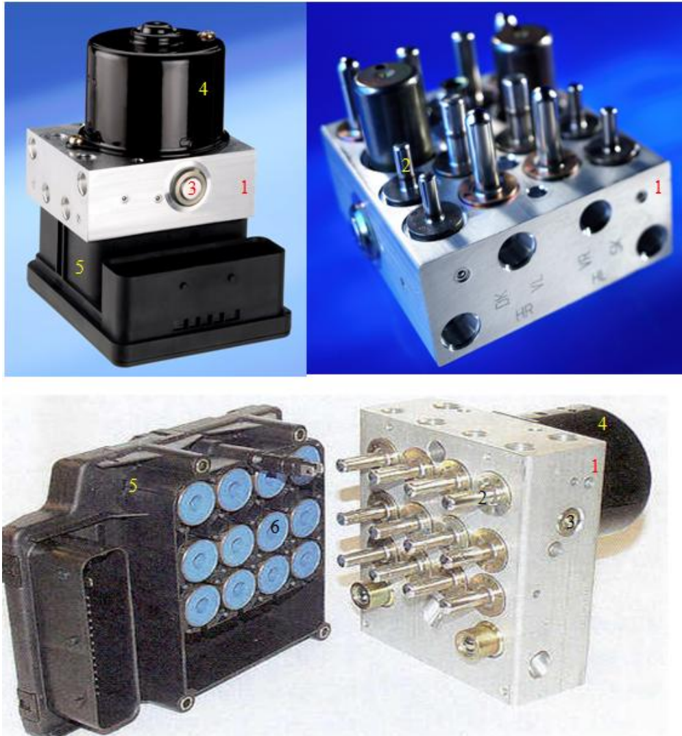
Figure 23 Continental Teves ® MK60 Brake Module. 1) Hydraulic block 2) Solenoid valves 3) Pump 4) DC motor for running the pump 5) Electronic control unit 6) Coils/solenoid group
