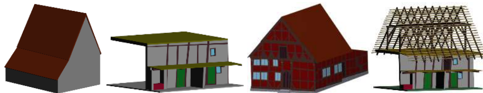
Figure 2. 3D model of Old-Segeberg town house: f.l.t.r. 1541 outside, 1541 inside, 1584-1588 outside and 1584-1588 inside
