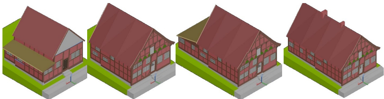
Figure 5. Advanced 3D models of the different construction stages of the town house. From left to right: 1541-1585, 1585 – ca. 1805, ca. 1805-1814 and 1814 – ca. 1890
