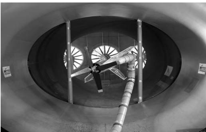
Figure 3. Vertigo model in elliptical test section.
