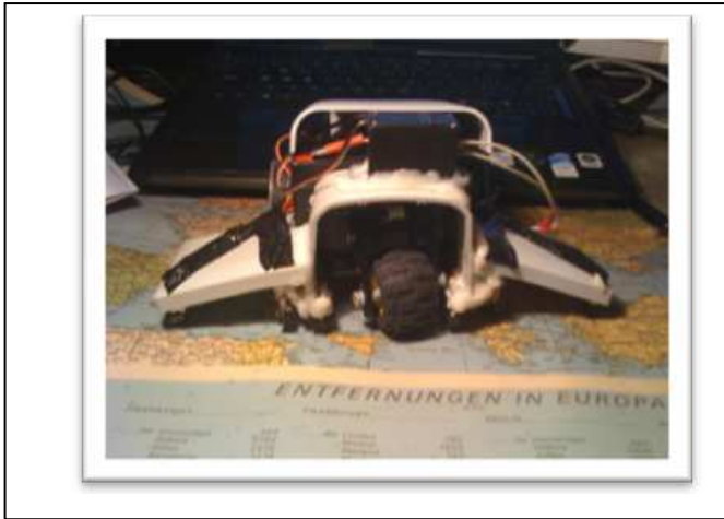
Figure 4. The robotic platform controlled by the gesture recogniser
