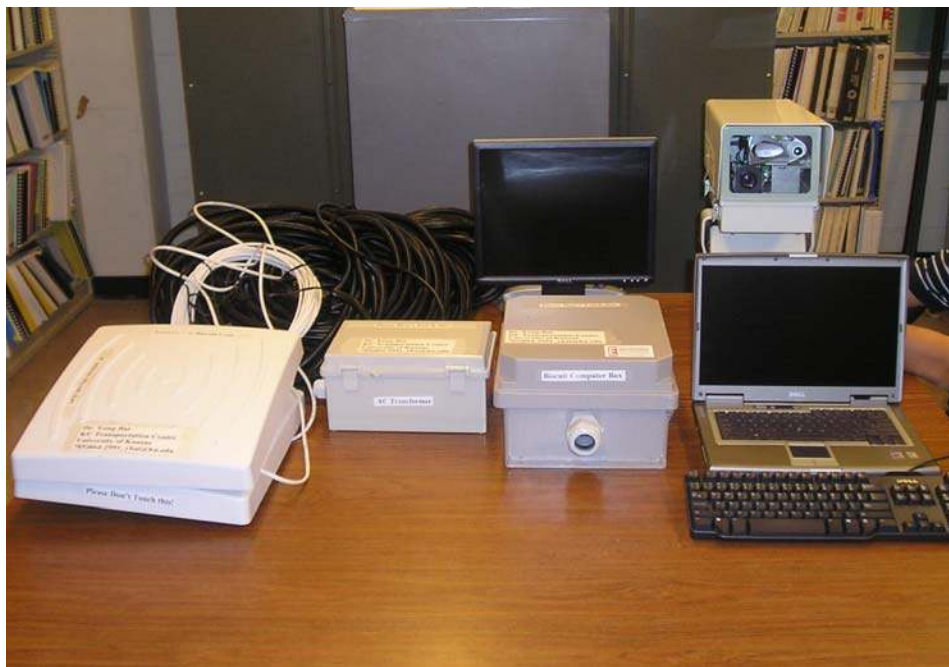
Fig. 11. Major components of the WRITE System
