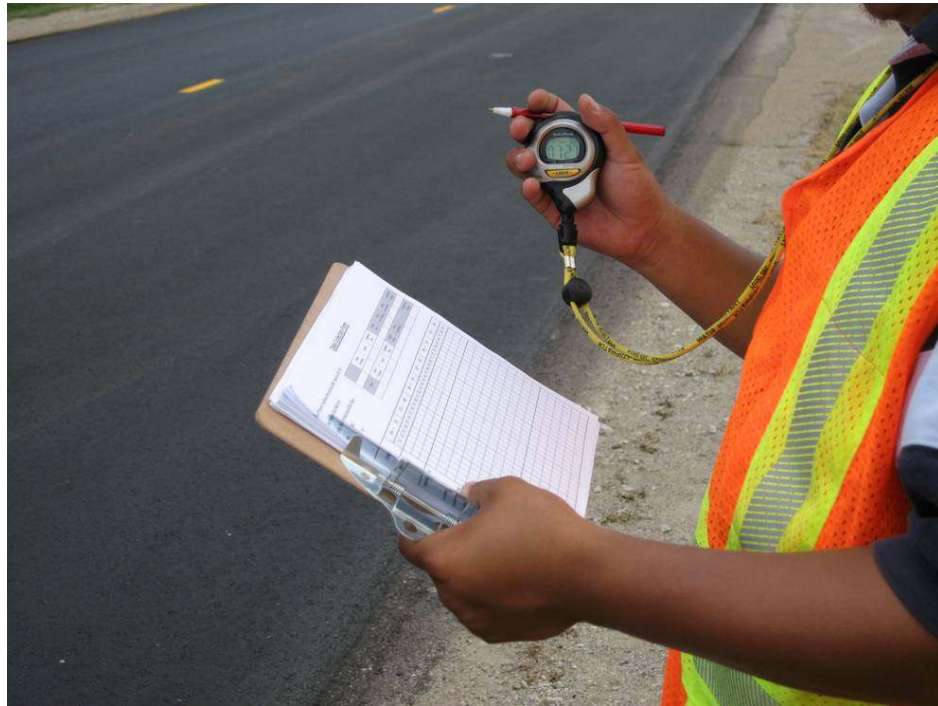
Fig. 35. Time study using stopwatch
