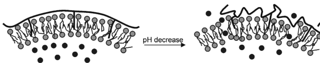
Fig. 7 Schematic representation of a possible mechanism for pH-triggered release by copolymers of NIPAM (adapted from ref. [73]).
