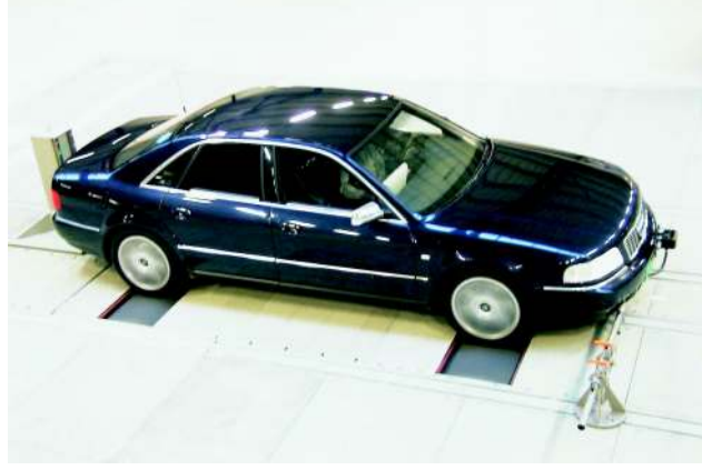
Figure 8. Vehicle under test with radar sensor at the front bumper, driving on the chassis dyno in VEHIL and supported by a rig at the front and back bumper.
