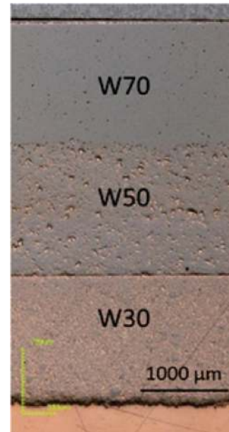
Figure 62. Micrograph of a W/CuCrZr composite interlayer after HHF loading up to 20 \text{ MW m}^{-2} (3 cycles).
