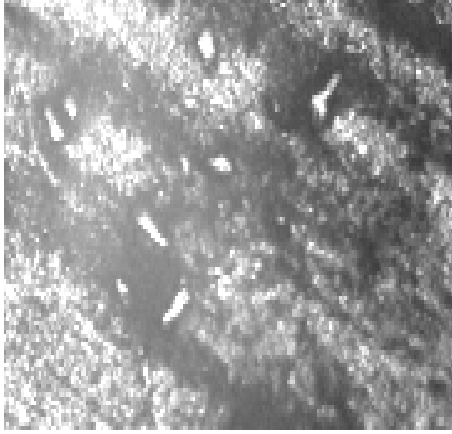
Fig. 10. Micrograph of sample containing 5% SiC by weight (100microns)
