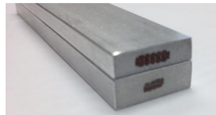
Fig. 3. DS1 and DS2 Al-stabilized cables after conforming and cold-work.
