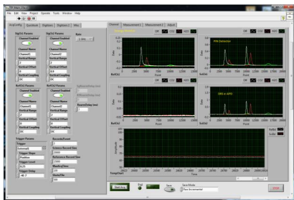
Figure 5 Data acquisition software GUI showing the triple-pulse energy monitor and return signals using InGaAs and MCT e-APD detection systems.
