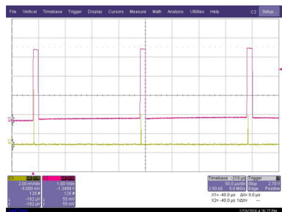
Figure 2 Single-shot temporal profile of the triple-pulse generation (yellow) as compared to Q-switch timing (red).
