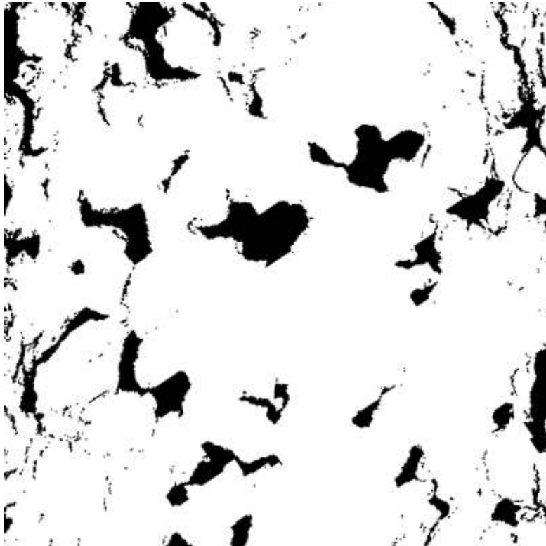
Figure 58: Resulting black and white image of the framed portion of the indented SEM image of Figure 57. This view is a planar projection of the actual cylindrical surface.
