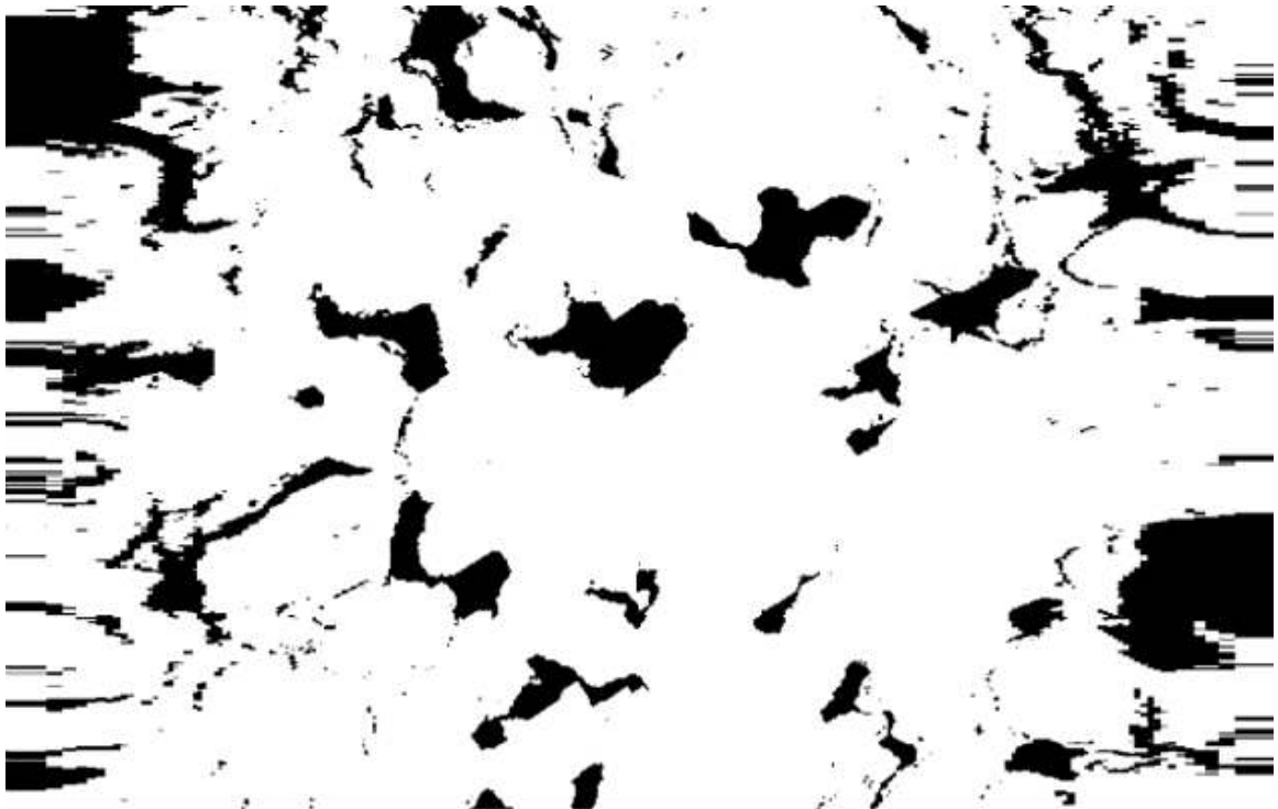
Figure 60: Unwrapped cylindrical projection of Figure 59 which appropriately removes the compression of the vertical side walls of the original image in Figure 58. Analysis of this view indicates a contact percentage of 83.2%.
