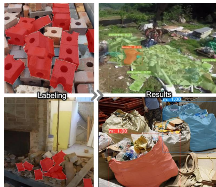
Figure 2. Labelling by applying instance segmentation to the collected construction waste images and the result of learning.
