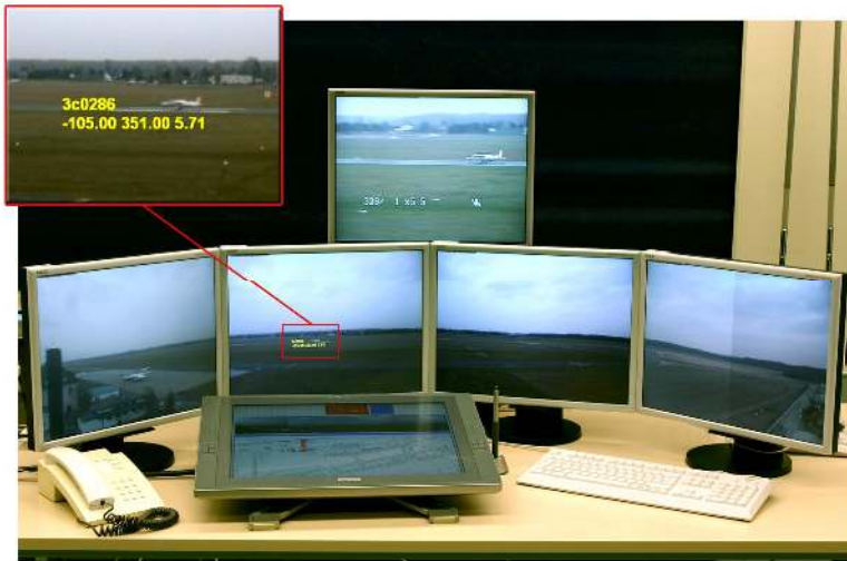
Fig. 4. Video panorama display system with additional PTZ display above (Photo:DLR)
