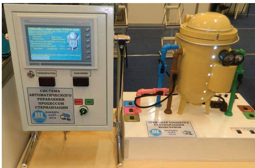
Figure 6: Sterilization process simulator model with control system.
